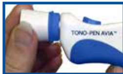
Position the Ocu-Film + applicator on the transducer.
