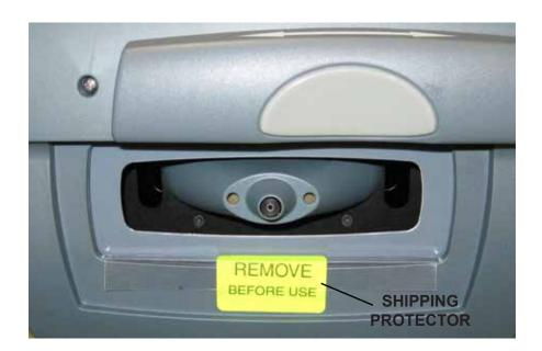
1. Pull the plastic Shipping Protector up and out of the opening on patient side of the instrument.
